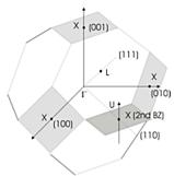
The figure on the left illustrates the first Brillouin zone of FCC lattice that corresponds to the first Brillouin zone for all diamond and Zinc-blende materials (C, Si, Ge, GaAs, InAs, CdTe, etc.). There are 8 hexagonal faces (normal to 111) and 6 square faces (normal to 100). The sides of each hexagon and each square are equal.
