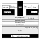
Schematic cross section of a High Electron Mobility Transistor (HEMT).
