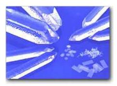
The arrangement of the atoms in a solid is broken down into three classifications: amorphous, polycrystalline, or crystalline. Silicon is the most common semiconductor material being used today because it the most abundant and can be found in all three arrangements.
