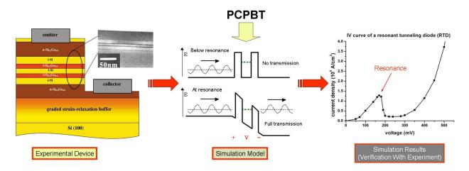
By completing the Piece-Wise Constant Potential Barriers Tool Lab (PCPBT Lab) in <u>ABACUS</u> - <u>Assembly of Basic Applications for Coordinated Understanding of Semiconductors</u>, users will be able to understand a) the concept of quantum-mechanical transmissions and reflections, b) a double-barrier structure and the concept of quasi-bound states, and c) the formation of energy bands due to the interation between the wells in a multi-well structure.
