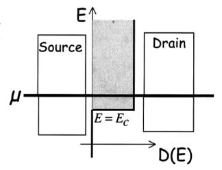
(a) Channel potential fixed with respect to source:  $\alpha = 0$ .
