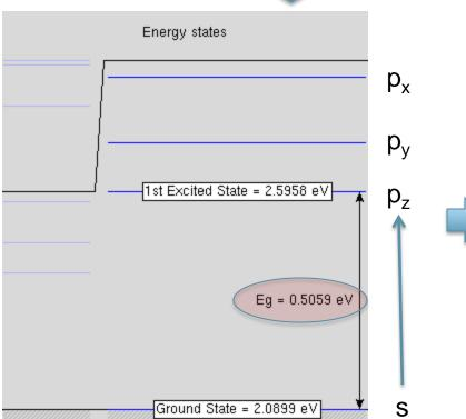
s to p<sub>z</sub> orbital transition can be observed by **Z-polarized light**
