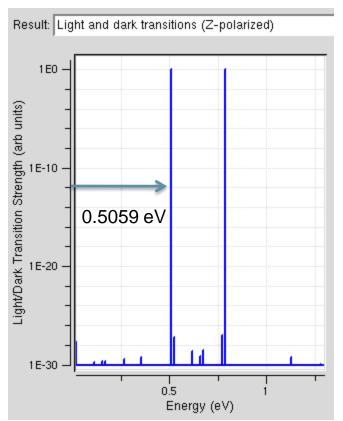
The first large transition comes exactly at the transition energy from s to p<sub>7</sub> type orbital.
