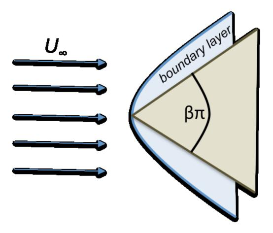
The general solution is called the Falkner-Skan boundary layer solution, which starts with a recognition that the free-stream velocity will accelerate for non-zero values of \$\$\beta\$:
