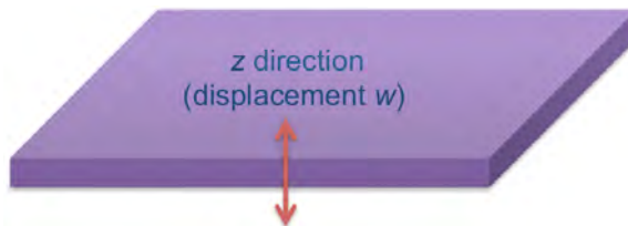
Fig. A.2 Schematic showing the vibrational displacement direction of the flexural mode of a thin plate.
