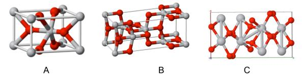
Figure 2. Representations of the crystal unit cells of titanium dioxide. (A) rutile, (B) anatase, (C) brookite. *Images from www.labspaces.net, Wikimedia Commons, and http://materials.springer.com.*
