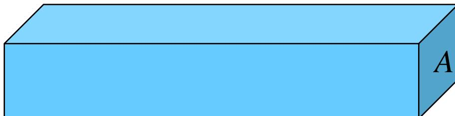
$$R_{3D} = \rho_{3D} \frac{L}{A} \quad \rho_{3D} = \frac{1}{n q \mu_n}$$
