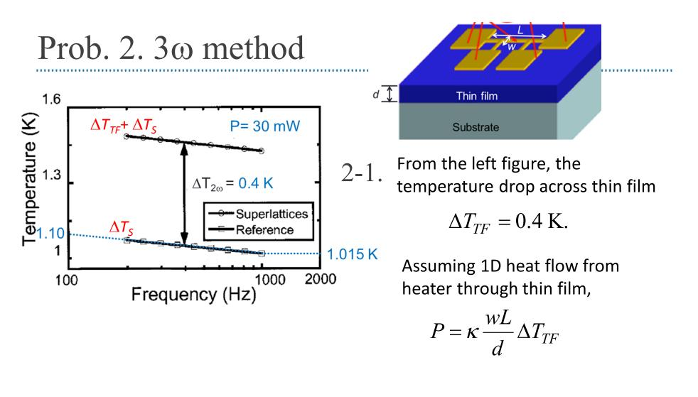
$$\therefore \kappa_{TF} = \frac{Pd}{wL\Delta T_{TF}} = \frac{(0.03 \text{ W})(1 \times 10^{-6} \text{ m})}{(25 \times 10^{-6} \text{ m})(1 \times 10^{-3} \text{ m})(0.4 \text{ K})} = 3 \text{ W/mK}$$
