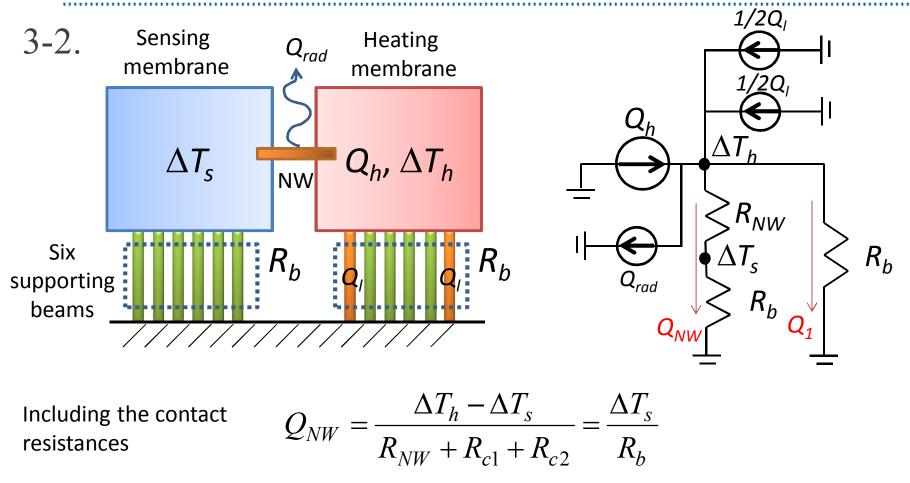
$$\therefore R_{NW} = R_b \frac{\Delta T_h - \Delta T_s}{\Delta T_s} - R_{c1} - R_{c2}$$
