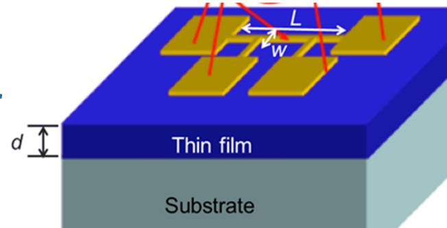
2-1. From the left figure, the temperature drop across thin film
