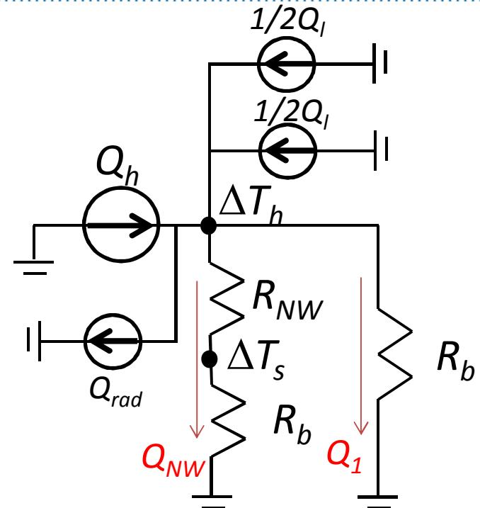
$$Q_{NW} = \frac{\Delta T_h - \Delta T_s}{R_{NW}} = \frac{\Delta T_s}{R_b} \quad Q_1 = \frac{\Delta T_h}{R_b}$$
