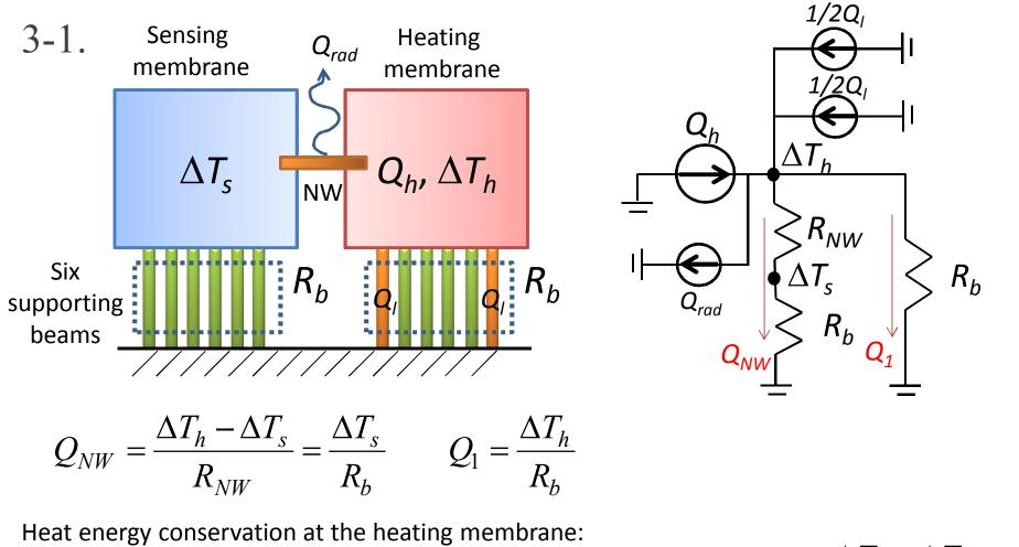
$$Q_h + Q_l - Q_{rad} = Q_{NW} + Q_1 = \frac{\Delta T_s}{R_b} + \frac{\Delta T_h}{R_b} \implies \therefore R_b = \frac{\Delta T_h + \Delta T_s}{Q_h + Q_l - Q_{rad}}$$
