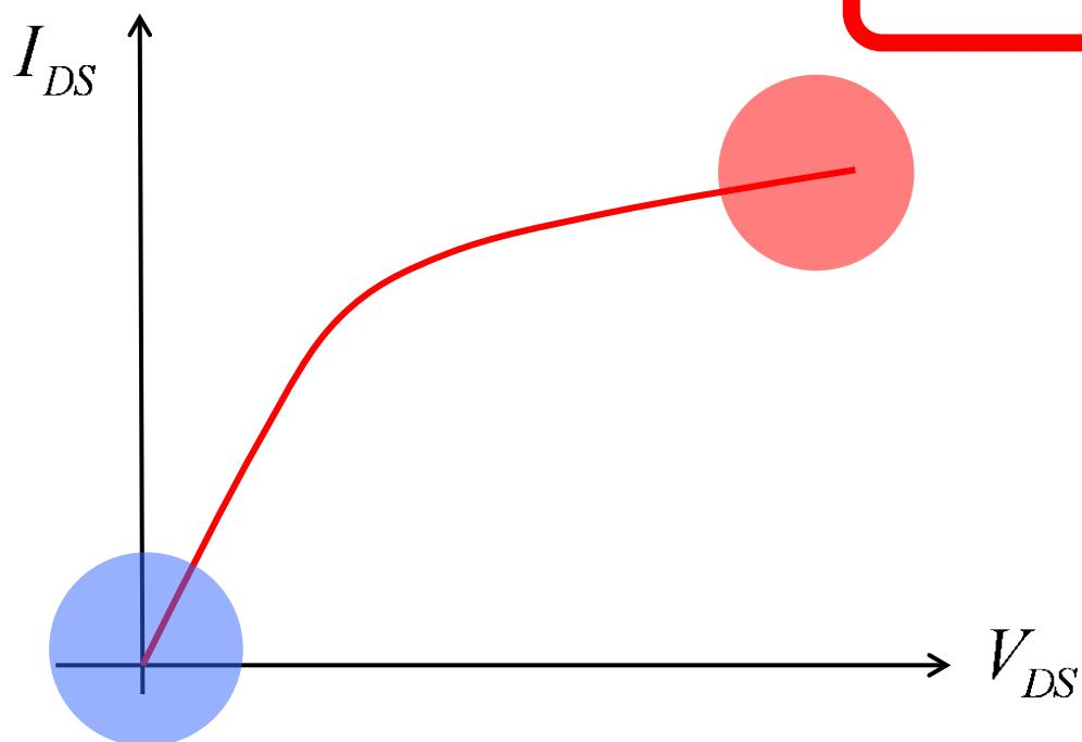
$$I_{DS} = W C_{inv} (V_{GS} - V_T) v_T$$
