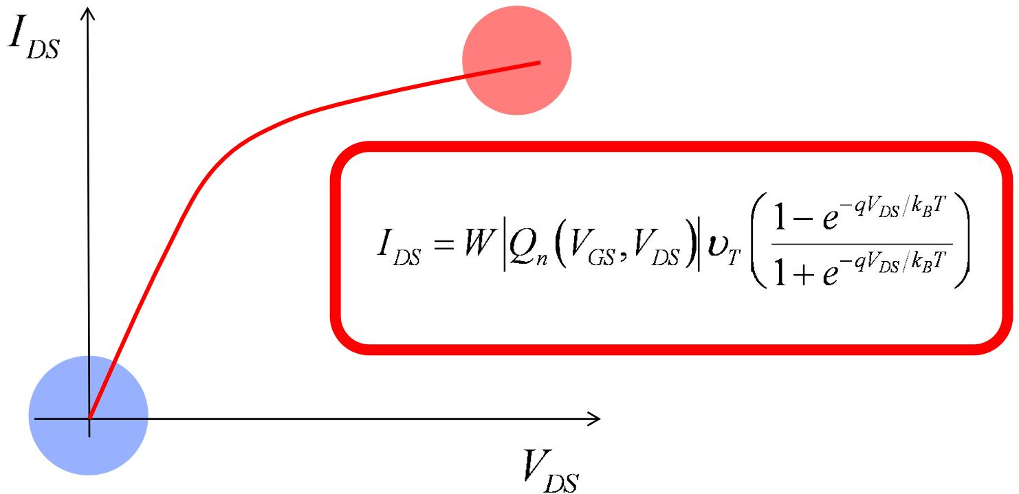
$$I_{DS} = W \frac{v_T}{2k_B T/q} |Q_n(V_{GS}, V_{DS})| V_{DS}$$
