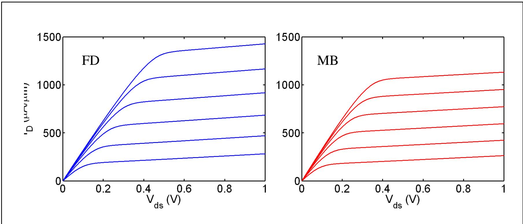
Ballistic calculations using typical numbers for an ETSOI MOSFET. By Xingshu Sun, in *Fundamentals of Nanotransistors*, Lecture 13, World Scientific, 2015.
