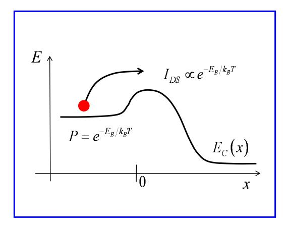
injection of thermal carriers over a barrier
