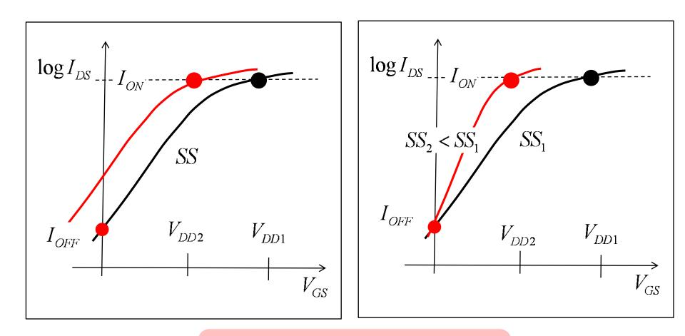
$I_{ON} \propto (V_{DD} - V_T) \quad I_{OFF} \propto e^{-V_T/k_B T}$
