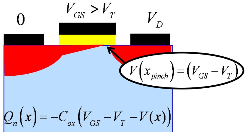
$$I_{DS} = -W Q_n(x) \langle v_x(x) \rangle = W Q_n(0) \langle v_x(0) \rangle$$
