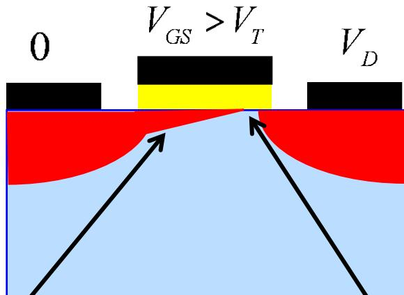
$$Q_n(x) = -C_{ox}(V_{GS} - V_T - V(x))$$
