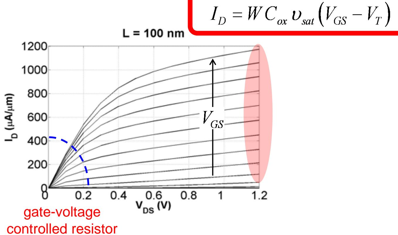
$$I_D = \frac{W}{L} \mu_n C_{ox} (V_{GS} - V_T) V_{DS}$$
