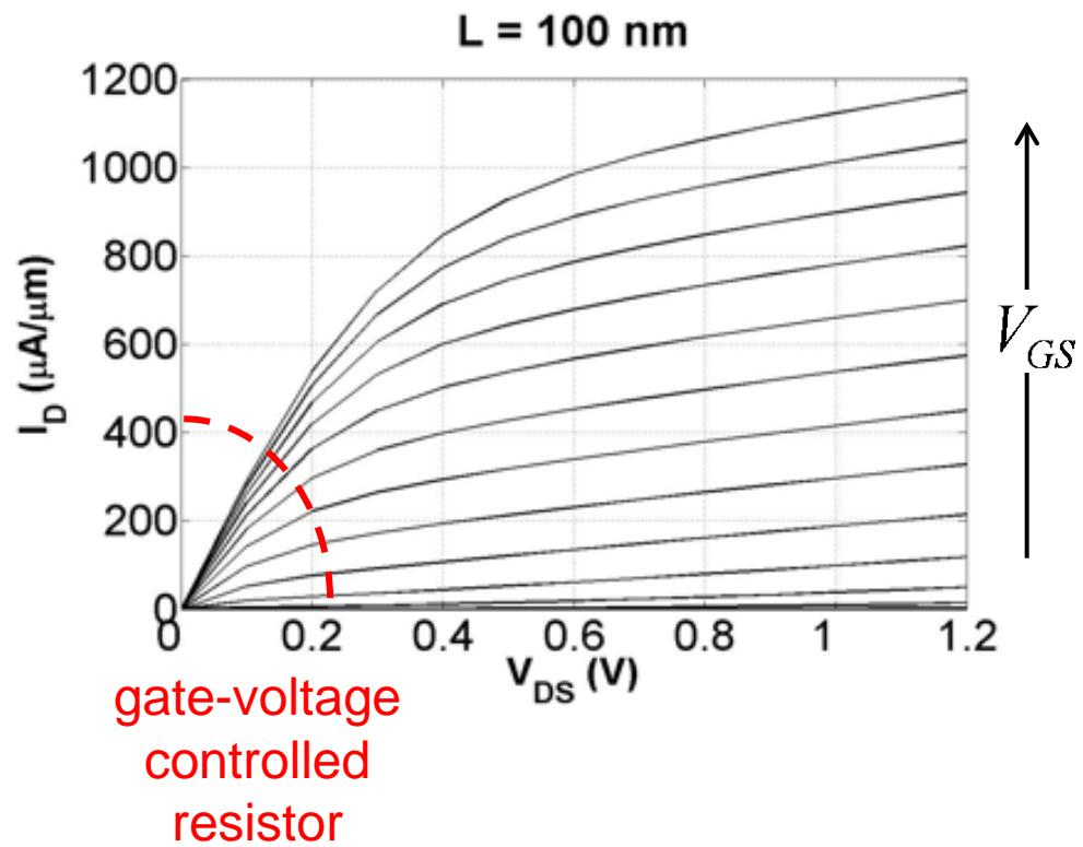
$$I_{DS} = \frac{W}{L} \mu_n C_{ox} (V_{GS} - V_T) V_{DS}$$
