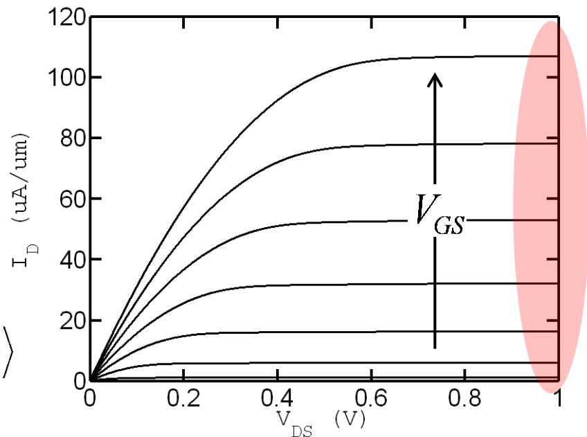
$$I_{DS} = \frac{W}{2L} \mu_n C_{ox} (V_{GS} - V_T)^2$$
