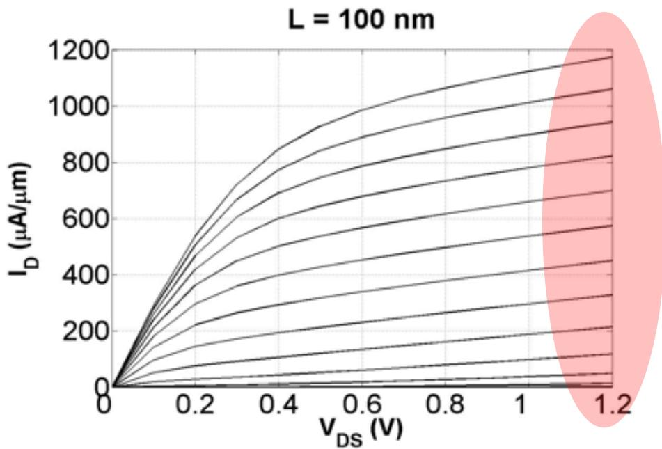
$$I_{DSAT} \propto (V_{GS} - V_T)$$
