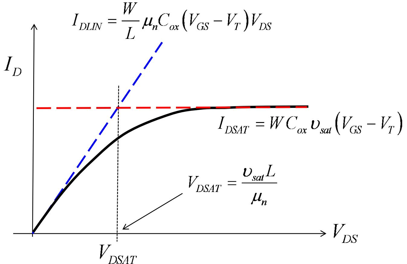
We have developed a 2-piece approximation to the MOSFET IV characteristic.
